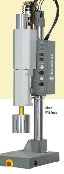
fabricated from high performance engineering resins, can be effectively welded at 15 kHz.
